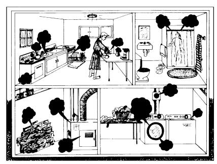
Figure 2.—Common indoor moisture sources.
