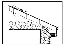
*Figure 5.*—*Passive attic vents.*
