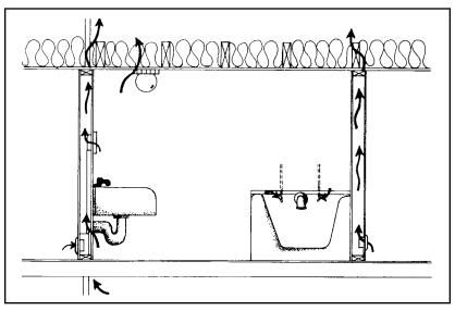
*Figure 3.—Attic bypasses from the bathroom.*
