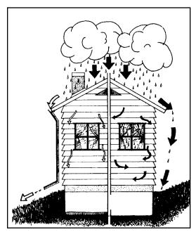
Figure 1.—Gutters, a slope away from the house, and drainage tile in the foundation keep the left side of this house dry. No gutters, a slope toward the house, and no drainage tile expose the right side to moisture damage.
